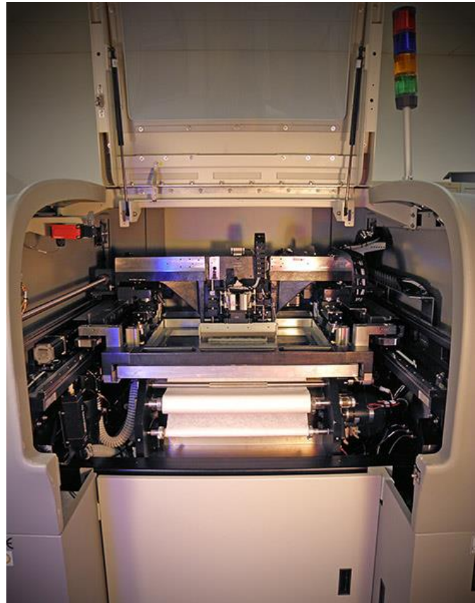
Figure 1. MPM Edison printer with 15-second throughput.
