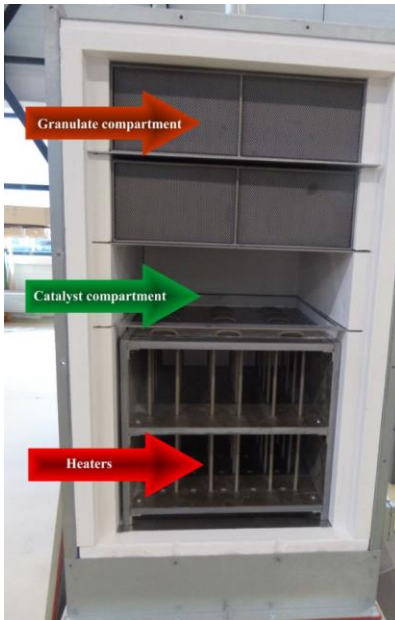
Figure 5 – the prototype, an universal collection unit with place for granulate as well as catalyst.
